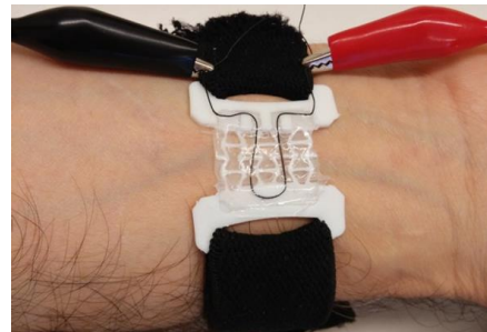
B) Elastomer band sensor worn on a wrist.
