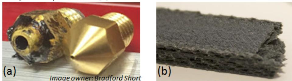
Figure 1: (a) Brass nozzle wear effect, (b) 3D printed Polyamide with 30% glass fibre
