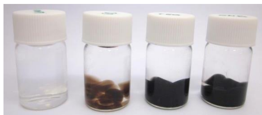
Figure 1 (from left to right): Photographs of bare hydrogel and hybrid hydrogels with GO, RGO and FLG (1 % wt.)
